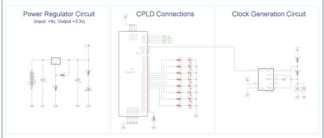
Putting the two capacitors in parallel makes the effect capacitance 0.2uF which creates a clock output to the CPLD of about 250 Hz. A good POV should run at about 100-150 Hz, so we'll divide it down by 2 inside of the CPLD.
