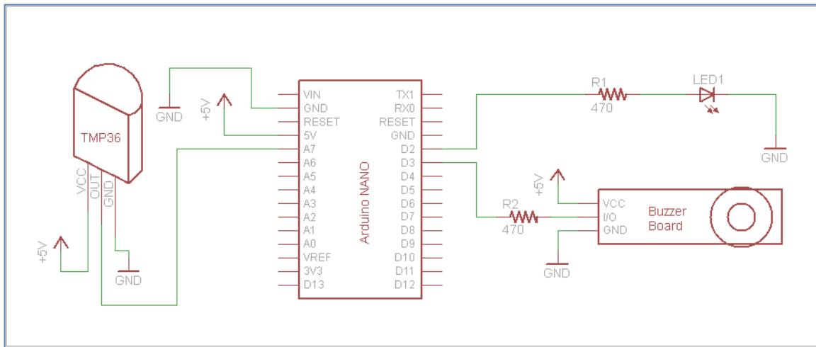
We start of this course with an easier project because in this lesson we also have to setup the arduino platform for development with the arduino nano. But still, this lesson is a good introduction into taking sensor input and setting an alarm's output.
