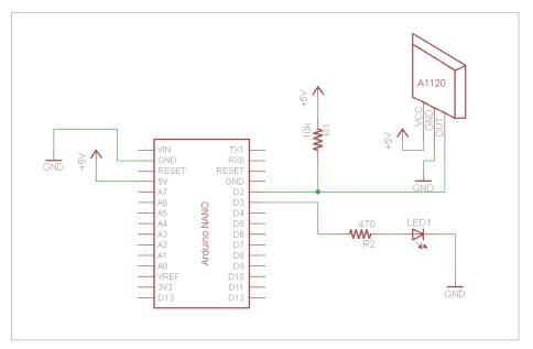
Whenever a magnetic field is detected near the hall effect sensor the red LED is turned on to visually notify us.
