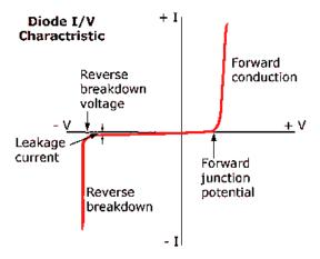
Diodes also have a breakdown state that you can see in the graph above. When enough negative voltage is applied to a diode, it can be forced on and allow electrical current to flow in the opposite direction; however this will most likely end with the diode being damaged.
