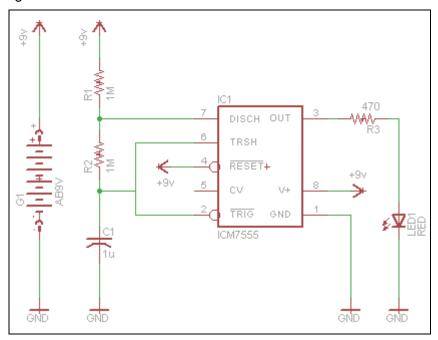
This is one of the more complex circuits that we built in this course but it was important to understand that we can easily control output signal timing by switching out resistor and capacitor components for larger and smaller values.
