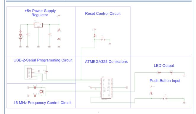
This is the schematic for the experiment in lesson 4. It uses a push button and an LED to represent how we can use the specific Arduino timing functions. These functions allowed our programs to perform pre-programmed actions at specific timing intervals.
