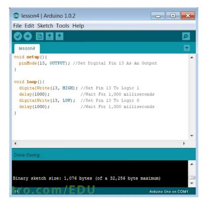
After a successful demonstration, we then changed the 1,000 inside of the delay() function to a 250, which made the LED blink much faster since the program pauses were then only 250 millliseconds.
