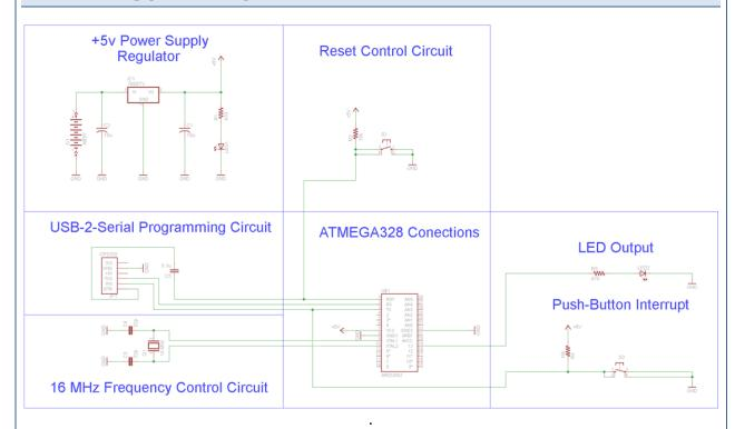
Here is the lesson 6 schematic. In this lesson's experiment, instead of using a polling technique to get input from the push button, we used an interrupt.
