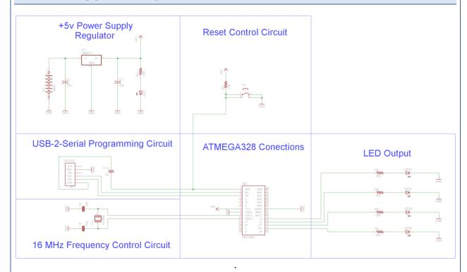
Here is the lesson 7 schematic. In this lesson we used serial communication to tell the ATMEGA328 microcontroller to turn on specific LEDs and then turn them off. A simple idea, but powerful once you realize that you can make two computer talk to each other!
