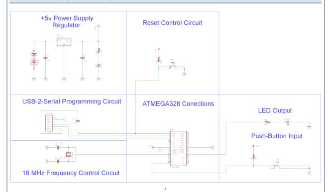
This is the lesson 3 hardware schematic where we added an LED to see output and used a push button to give input to the microcontroller. The schematic is very similar to the one we used in lesson 2 so no need to fear the hardware in it!
