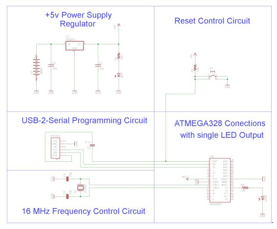
This is the complete hardware schematic for lesson 2 of the Introduction to Microcontrollers course. The 5 different unique sections are all important to get LED2 to turn on programmatically.
