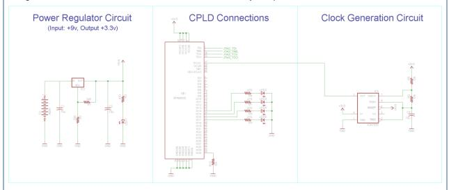
This circuit uses the ICM7555 timer to generate a +3.3v clock signal at a slow 10-15 Hz frequency for the CPLD to use as a timer. All power voltages used are +3.3v coming from the regulator circuit.
