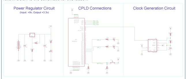
This schematic shows 1 input from a push buttons and 2 output to an LEDs all connected to the CPLD. The big new addition is the ICM7555 clock circuit, which outputs a 10-15 Hz clock signal to the CPLD.
