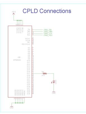
There are only 2 main components to this schematic: the power regulator circuit which takes +9v from a battery and regulates it to +3.3v output which our CPLD will use and the CPLD connections, where power and ground connect as well as the LED off of pin 22. The JTAG signals also need to be connected to the JTAG programmer in order to load the CPLD image.
