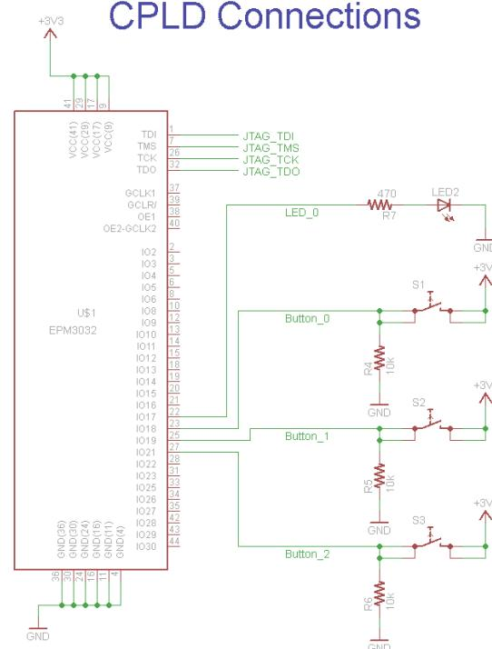
This schematic shows 3 inputs from push buttons and 1 output to an LED all connected to the CPLD.
