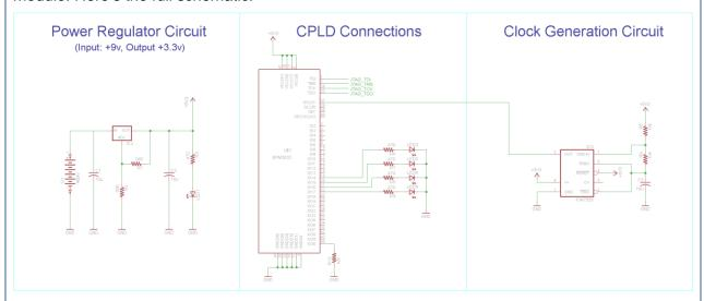
This schematic is virtually the same as lesson5, but we got rid of the push button and added a few extra LEDs to the mix.
