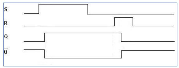
As you can see above, for a NOR gate SR latch, when the Set signal pulses to logic 1, the Q output sets to logic 1 and the Q\* output goes to logic 0. Similarly, when the Reset signal is pulsed with a logic 1, the SR latch resets the Q output to logic 0 and the Q\* output to logic 1.
