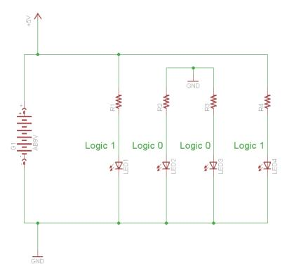
Really the schematic is just turning on some LEDs with the On-Off-Off-On pattern that matches the 1001 of binary. Translating 1001 to decimal we get the number 9.
