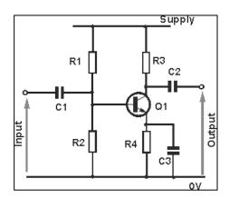
The second circuit above, on the right, is a more classical single transistor amplifier, with 4 resistors and 3 capacitors. The resistors allow a designer to properly 'bias' each point of the transistor amplifier and the capacitors allow for blocking DC and filtering out certain frequencies.
