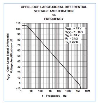
The graph makes it pretty obvious that right around 1 MHz we cross the 0 decibel power level which means no power gain from the input signal. This is called 'unity gain' and all opamps have this attribute which defines the upper frequency limit of input signals that they are able to amplify.
